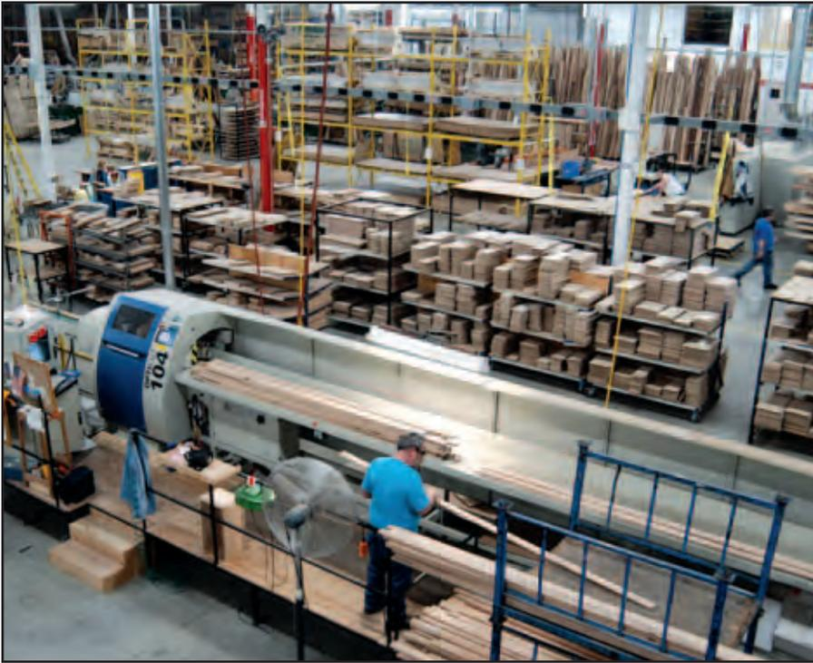
*Expansion of the Charles City Hardwood Facility provides for a bright, clean, efficient work area. The machine in the foreground automatically determines the most parts possible from a particular piece of wood, cuts those parts and sorts the cut pieces.*
