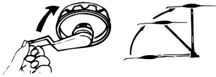
**Rotating Antenna** - Make sure antenna is in the “UP” position. Pull down on rotating knob until it disengages ceiling plate and rotate for best picture and sound on TV set.
