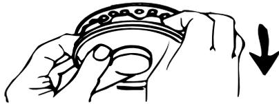
**Lowering Antenna to Travel Position** - Rotate antenna until pointer on rotating knob aligns with pointer on ceiling plate.
