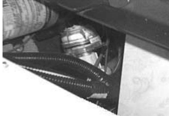
Models 22QD & 22HD: The shower pump is located beneath the wardrobe cabinet and is accessible by lifting the left rear dinette seat as shown in the photo below.
