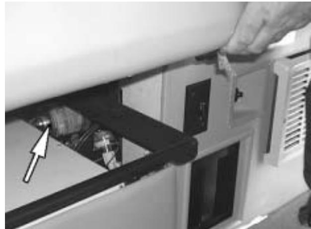
Model 22FD: The shower pump is located below an access hole beneath the bedboard at the foot of the rear bed in the left (driver side) rear of the coach.
