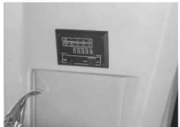
**Model 22QD:** The monitor panel is located on the wall near the left rear dinette seat. Press the corresponding buttons to test levels of the water tank, holding tanks. LP gas tank and battery condition. There is also a water pump
