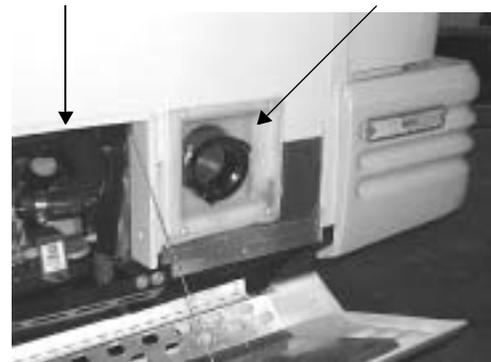
1. Remove drain hose from hose compartment.
