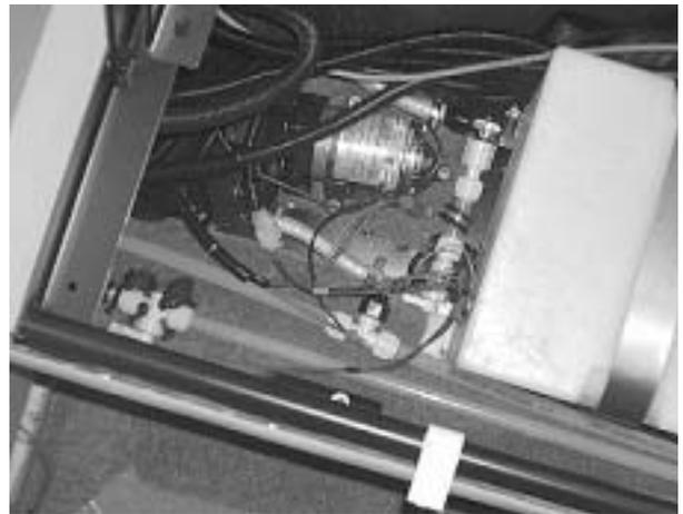
The panel is held in place against the seat frame tubes by strips of hook-and-loop tape.
