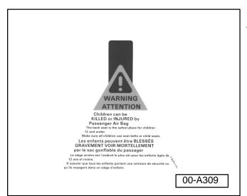
■WARNING! label, when installed, must be attached inside at the center of windshield, the bottom edge of the label must touch the top of the instrument panel such that the label itself is not curled or bent.
