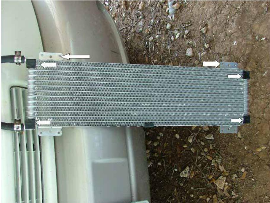
17. Cooler in place. End of hose clamp bent straight up to prevent contact with power steering cooler tube. I later added more padding at the top of the cooler fitting (arrow) to keep the hose clamp from touching.
