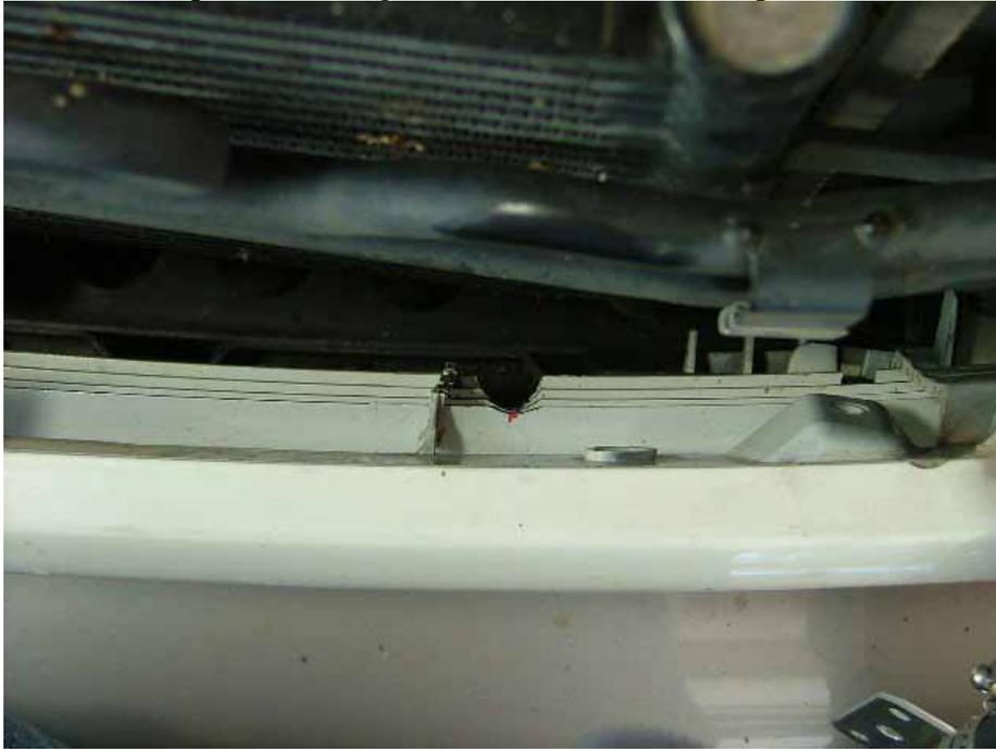
14. Lower hose attached to the cooler and temporarily installed to check clearance.
