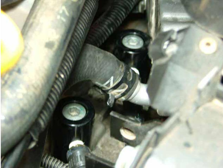
12. Hose routing beside the radiator to the front. I later added some of the split plastic tubing over the hoses to keep them from rubbing on the metal around the corners. Exact routing to the gap isn't critical, but avoid sharp turns and metal edges.
