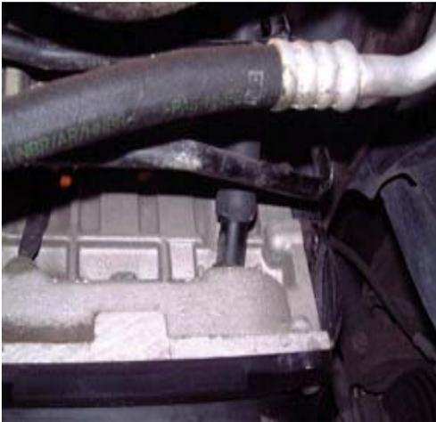
*Heater hose inserted over the short filler tube.*
