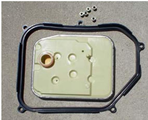
*The Transmission pan gasket and the transmission filter with filter gasket installed. (Also note the metal spacer sleeves that go in the gasket bolt holes.)*
