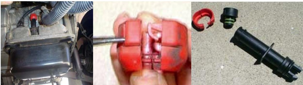
*The fill tube in place on the transmission.*      *The seal opens when the catch is released.*      *The three components of the fill tube assembly.*
