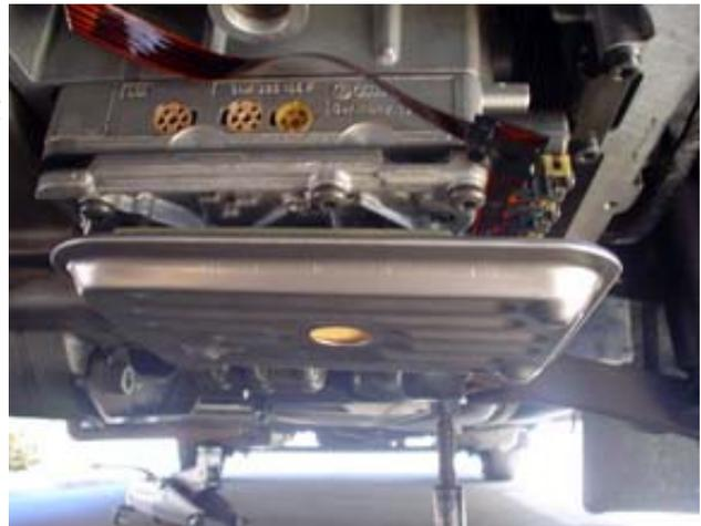
13. (a) **67 percent replacement** – reinstall the overflow tube and use the 5-mm Allen key *The new filter in place* to carefully hand-tighten it, bearing in mind that it's only plastic, and then reinstall the overflow plug and tighten with the Allen key.
