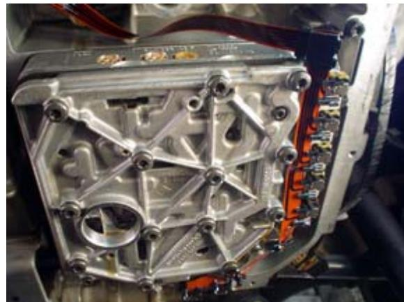
*Underside of the transmission with the pan and the filter removed.*
