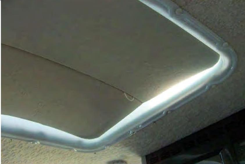
Built of .25" thick Styrofoam panels, with Reflectix on the top, and bonded fabric on the underside, it folds to store. Two panels 13 3/8" x 25 3/8" with 2.25" corner radius, are easy to build. Matching fabric is bonded to the side you can see and goes up around all edges to bond to the top of the Reflectix. A strip of 2" wide duct tape serves as a hinge on the top center
