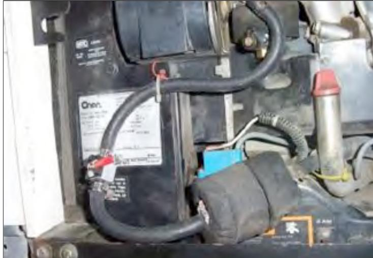
This simple modification prevents the build up of varnish and gum in the generator carburetor, which may occur when the generator is not used for more than a month. A metal valve is placed in the fuel line for the generator, in order to shut off the fuel supply, so the generator may be run until the fuel is exhausted.
