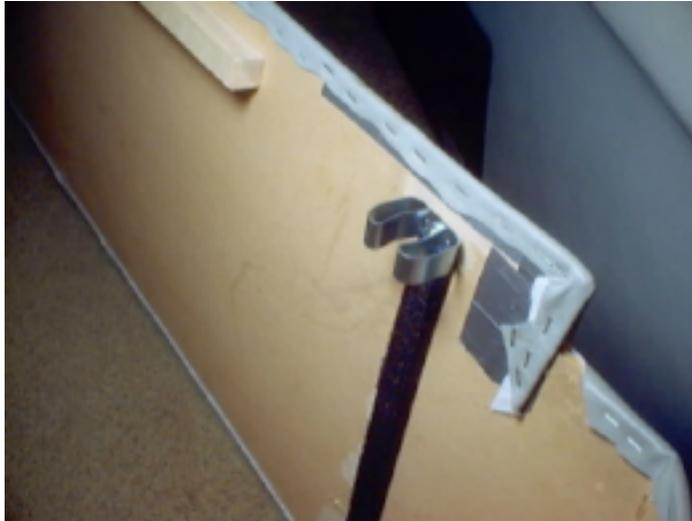
In the QD and HD models, the kick panel on the passenger's side that covers the fresh water tank is originally held in place by two strips of Velcro. Adding two grip clips makes it easier to remove and re-apply this panel and so makes it easier to confirm the amount of water in the fresh water tank and to store items on and around the tank.
