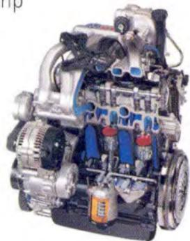
*The 1999 Rialta is equipped with a 2.8 liter VR6 engine.*
