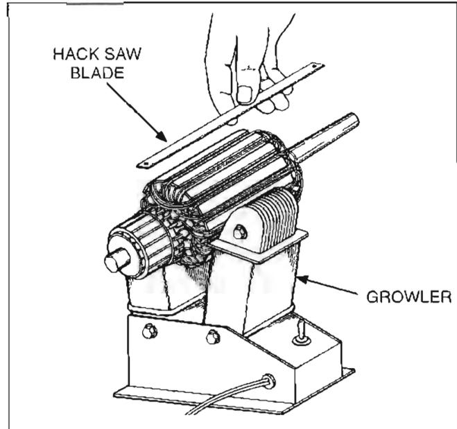
FIGURE 8-31. TESTING ARMATURE FOR SHORTS
