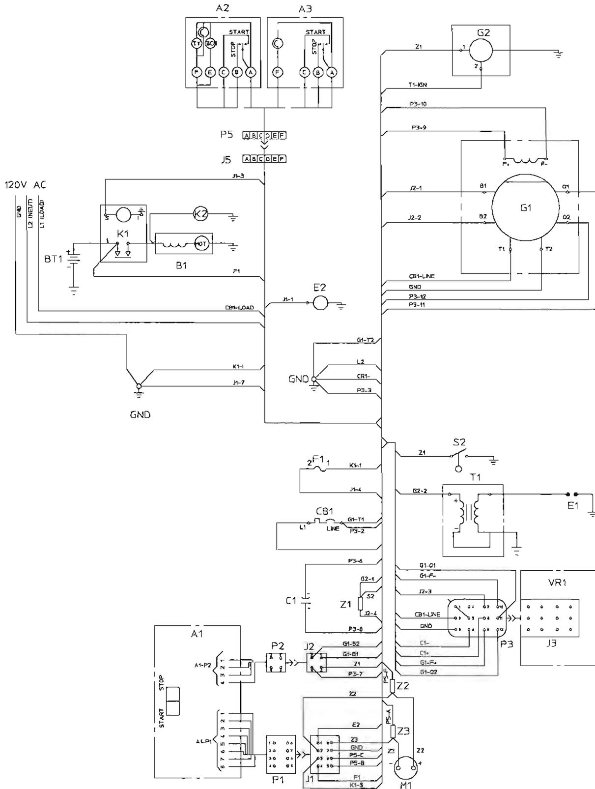
FIGURE 12-12. WIRING DIAGRAM 610-0395 (60 HZ) (KVC)
