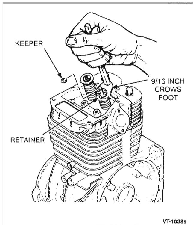
FIGURE 10-6. VALVE REMOVAL
