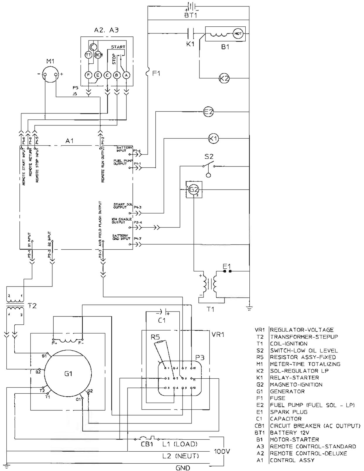
FIGURE 12-13. WIRING SCHEMATIC 610-0396 (50 HZ) (KVC)
