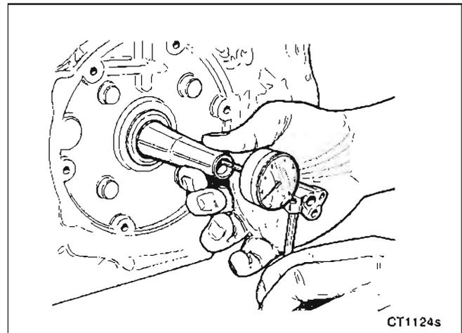
FIGURE 10-26. CHECKING ENDPLAY
