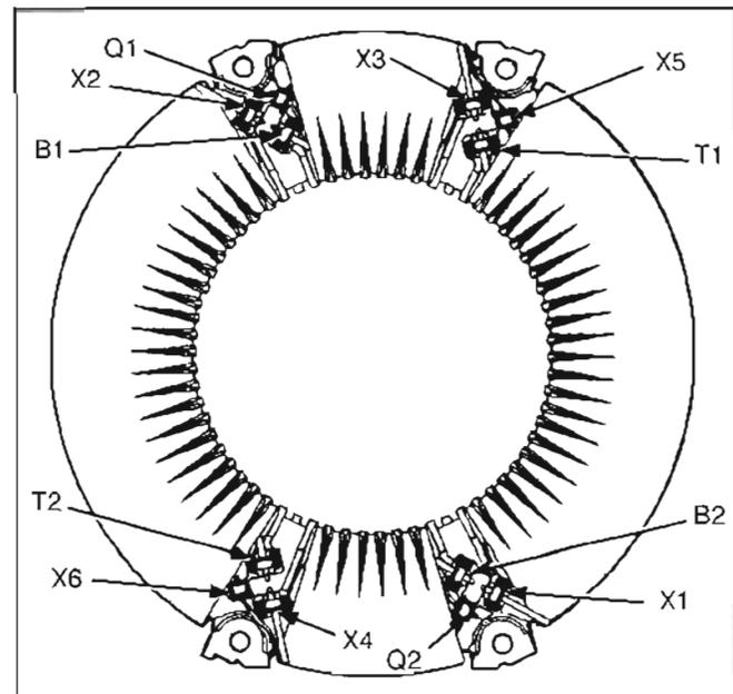
FIGURE 9-6. STATOR ASSEMBLY
