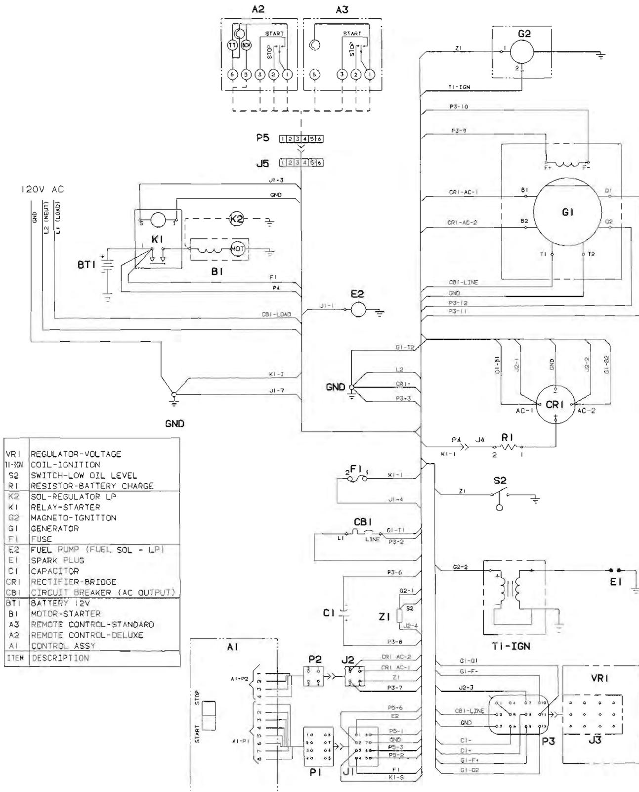
FIGURE 12-2. WIRING DIAGRAM 610-0382
