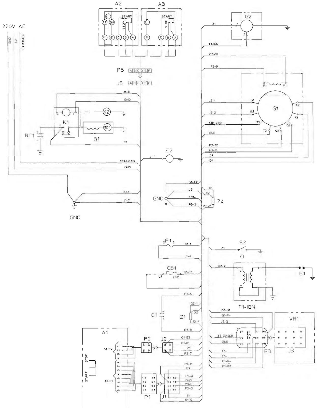
FIGURE 12-10. WIRING DIAGRAM 610-0389 (50 HZ) (BEGIN SPEC F)
