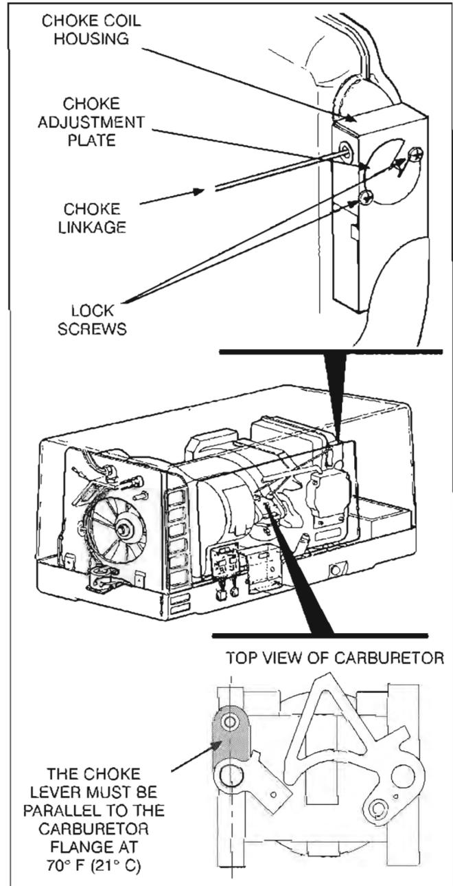
FIGURE 8-23. CHOKE ASSEMBLY (TYPICAL ALSO OF MODEL KVC)
